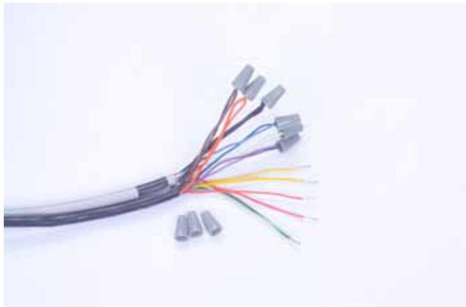
Splicing cable with wire nuts
